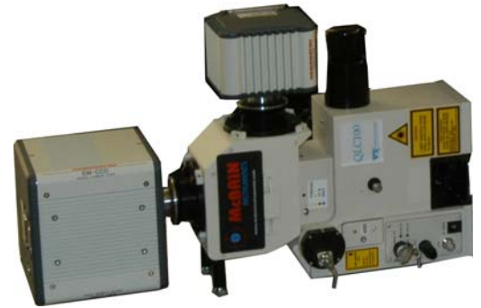
Yokogawa QLC100 scanning head with dual camera port adapter
