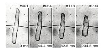
The images are taken with a pco.inspector hs from a sequence showing the punching action of a machine with a backswing that caused errors in the process. After having seen the sequence, the problem had been solved (1280x1024pixel, 636fps).
