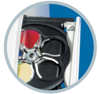
Filter wheel with five filter positions: Change of the wavelength range of the light with just a turn of the wheel.
